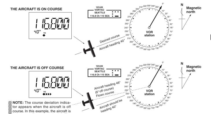
tor appears when the aircraft is off course. In this example, the aircraft is 6 degrees off course to the left. The pilot must turn more than 6 degrees
