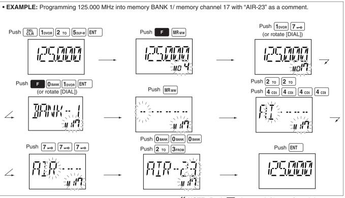
NOTE: Push , then push [0•BANK], and then rotate [DIAL] to select the BANK number, if desired. Push [CLR•DEL] to exit the BANK selection mode.
