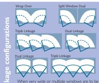
When very wide or multiple windows are to be swept we offer a comprehensive range of swept area solutions utilising the 70Nm drive unit operating either two or three arms and blades off one motor.
